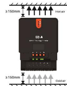
Fig. 2.1 Installation and heat dissipation
